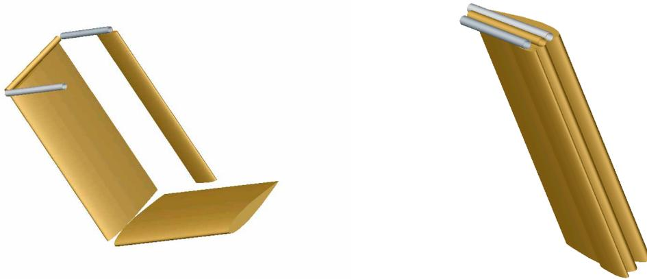
**Figure 6-4 Potential TCS wing assembly foldings**
