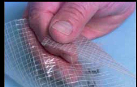
Composite Mars balloon material
