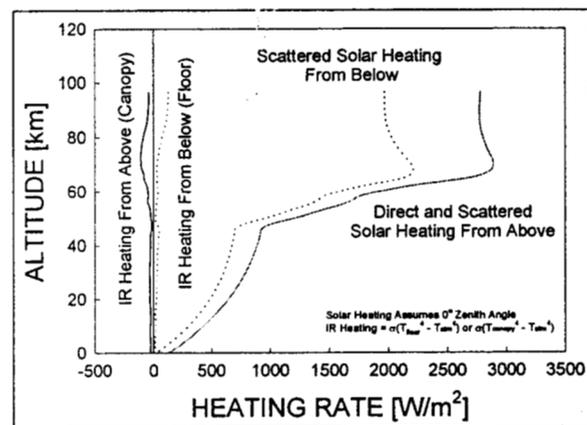
Figure 4: Solar heating from both direct and scattered sources (from below and above gondola).
