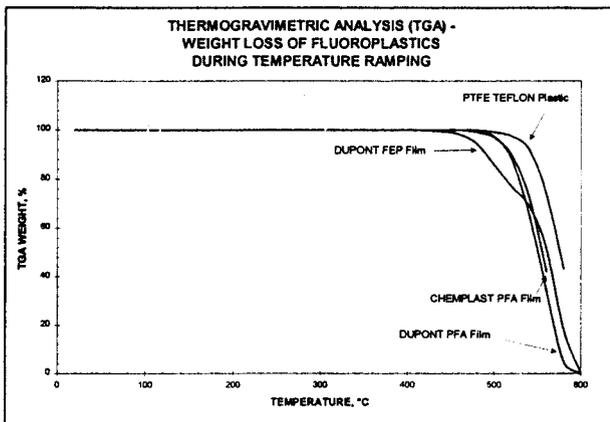
Figure 23: Thermogravimetric analysis of fluoroplastics during temperature ramping.
