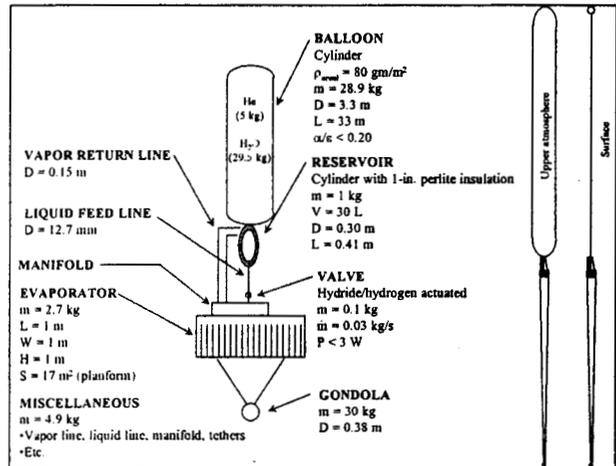
Figure 8: Buoyancy system configuration.
