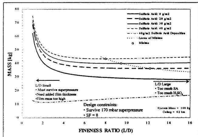
Figure 15: Effect of fineness ratio (L/D) for various sulfuric acid droplet density values.
