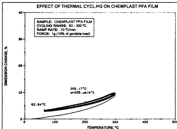
Figure 24: Effect of thermal cycling on chemplast PFA film.
