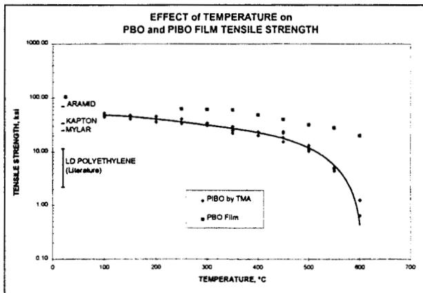
Figure 18: Temp vs. PBO/PIBO tensile strength.
