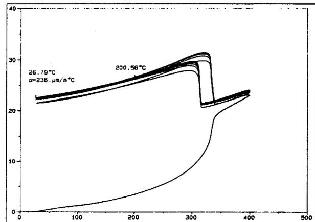
Figure 25: Temperature cycling of PFA.
