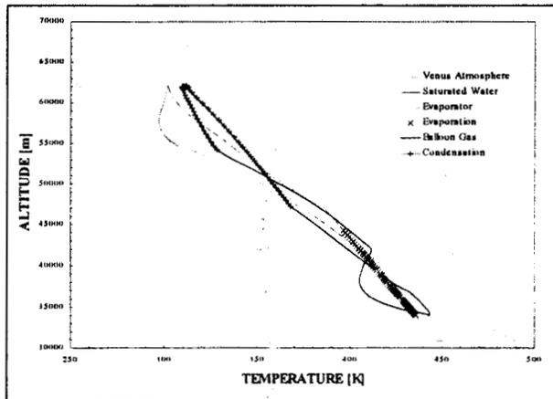
Figure 17: PCF Evaporation and Condensation Physics
