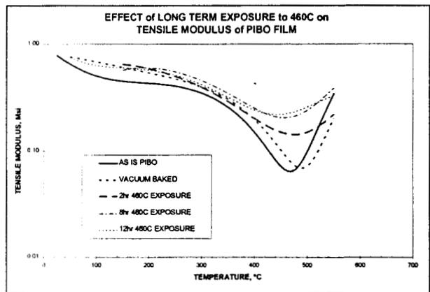
Figure 21: Long term exposure to 460C, PIBO film.
