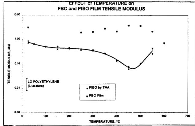
Figure 19: Temp vs. PBO/PIBO tensile modulus.
