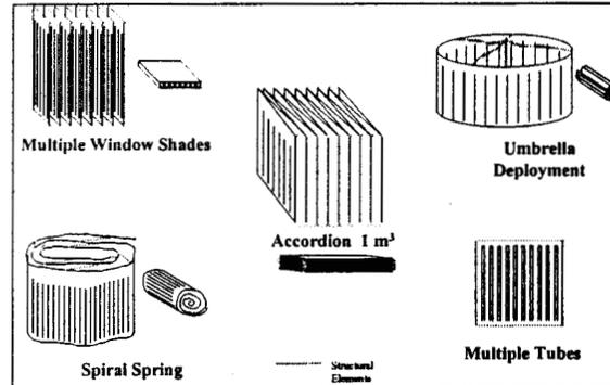
Figure 13: Evaporator configuration design options.
