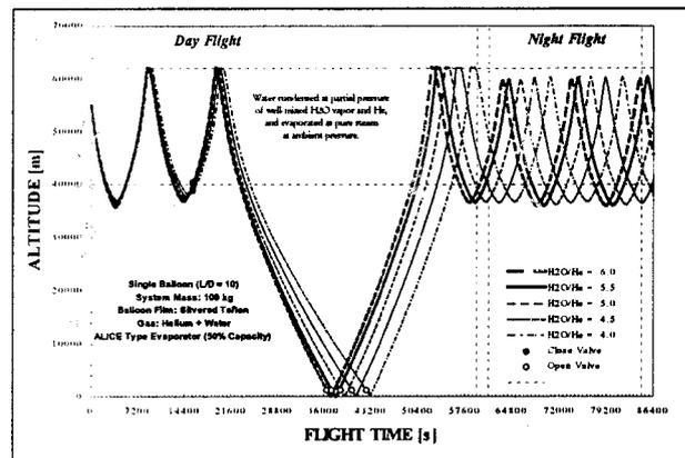
Figure 11: Effect of mixture ratio for the baseline helium/water mixture.
