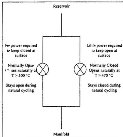
Figure 12: Dual-valve system diagram.
