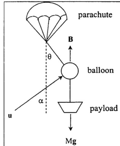
Figure 28: Deployment static stability diagram.
