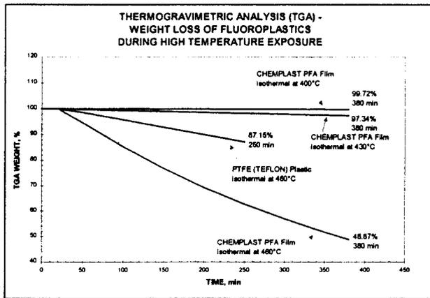
Figure 22: Thermogravimetric analysis of fluoroplastics during high temperature exposure.
