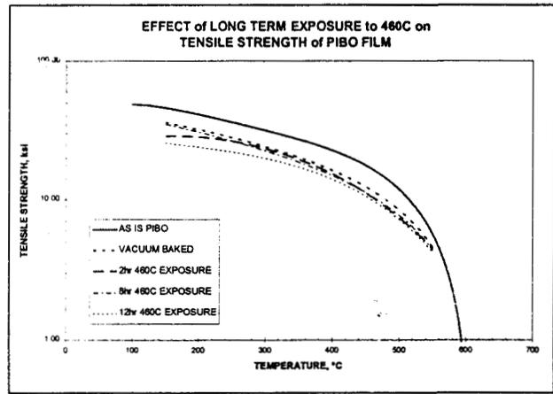
Figure 20: Long term exposure to 460C, PIBO film.
