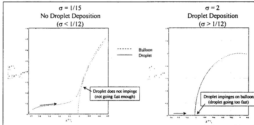
Figure 14: Representative droplet trajectories.
