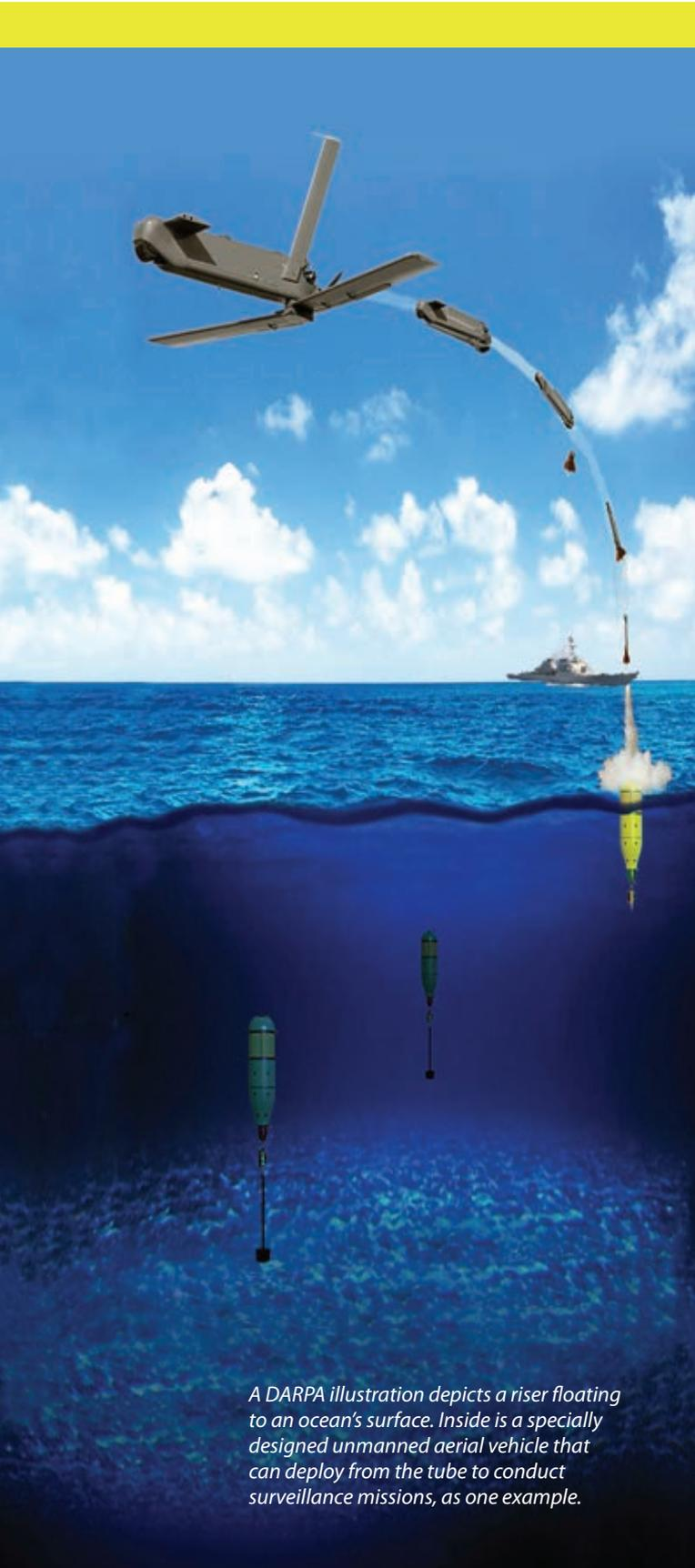
*A DARPA illustration depicts a riser floating to an ocean's surface. Inside is a specially designed unmanned aerial vehicle that can deploy from the tube to conduct surveillance missions, as one example.*
