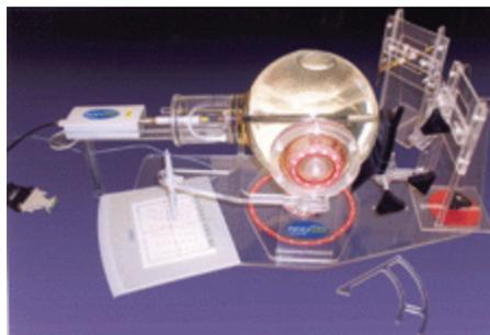
*MapSAR equipment is designed to measure how far radio frequency radiation from cellular phones absorbs into brain tissue.*
