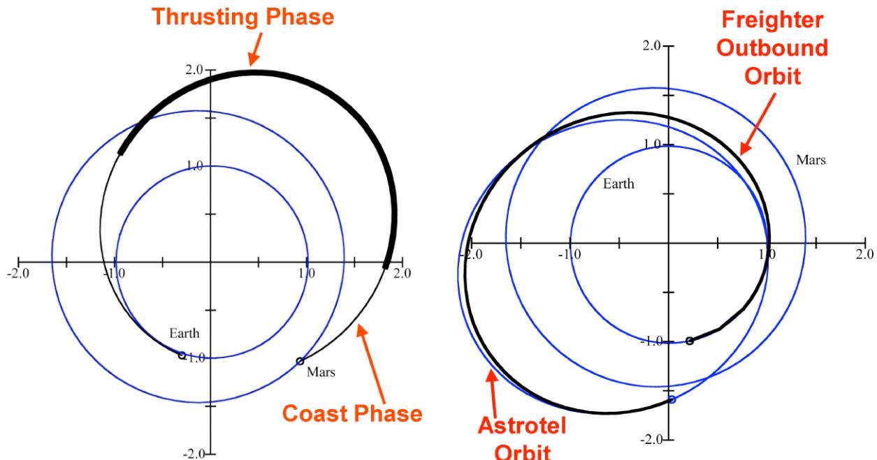
**Figure 6 Low-Thrust Maneuvering on Orbits.** The left set of orbits illustrates the Astrotel low-thrust orbit shaping and the right set of orbits illustrate the Astrotel Cargo Freighter low-thrust maneuvering and rendezvous
