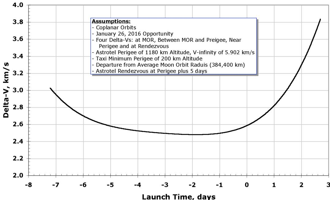
**Figure 5 Total Taxi delta-v as a function of launch time from the near-optimal time.**
