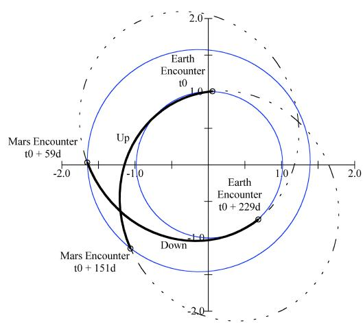
**Figure 3 Up and Down Escalator Resonant Orbits**
