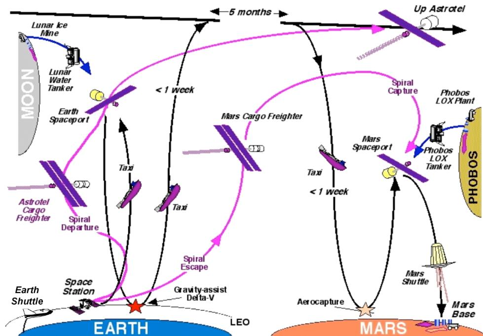
Figure 1. Overall concept of operations for the Earth to Mars flight profile.
