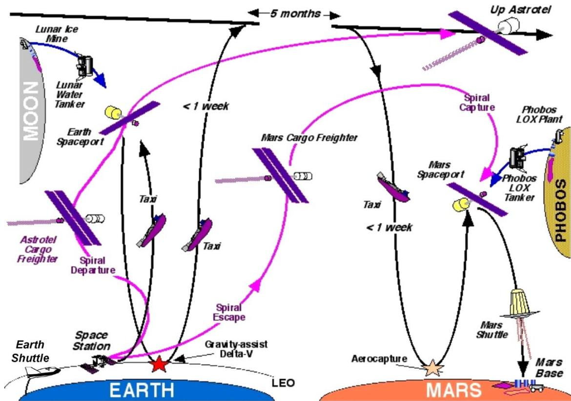
Figure 5. Overall concept of operations for the Earth to Mars flight profile.
