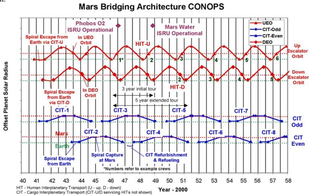
Figure 7 Mars bridging transportation architecture CONOPS Profile
