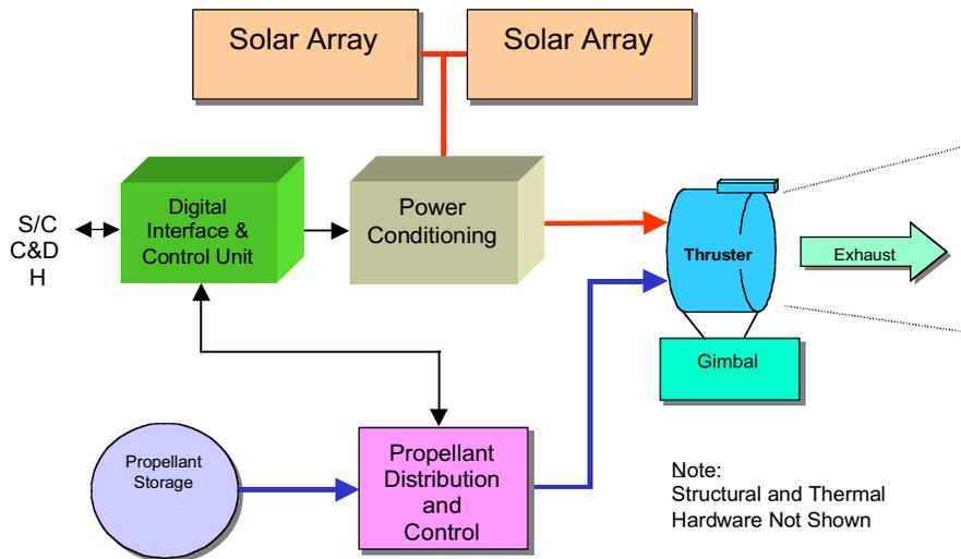
Figure 8-2 Simplified Block Diagram of an IPS (courtesy J. Brophy, JPL)
