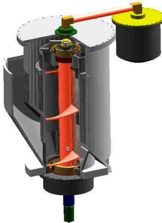
Figure 7-6: Lunar Ice Excavator Extractor.
