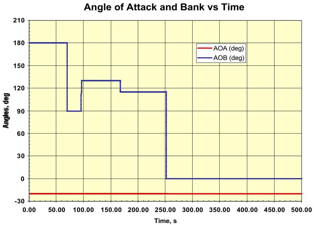
Figure 6-6 Taxi Mars Aerocapture Angle of Attack and Bank Angle Profiles
