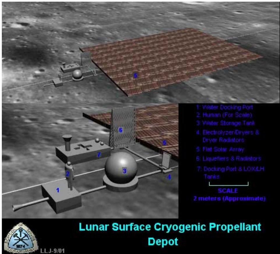
Figure 7-13 Lunar Polar Propellant Depot Rendered 3D Solid Model.
