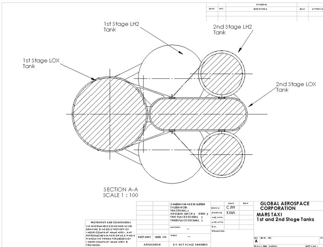
Figure 8-21 Line Drawing of Propellant Augmentation Tanks for 1st and 2nd Taxi Stages
