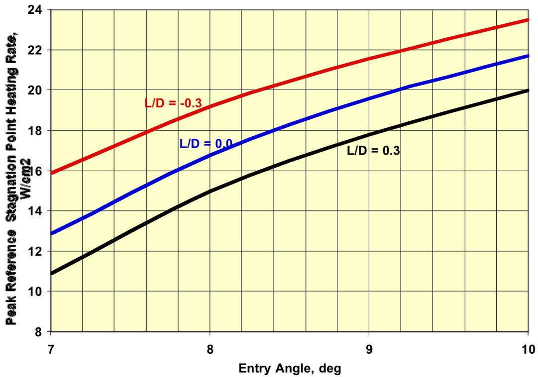
Figure 6-14 Peak Reference Stagnation Point Heating as a Function of Entry Angle
