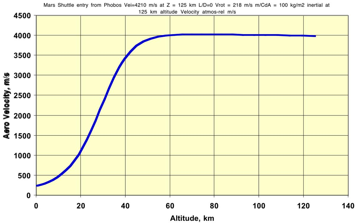
Figure 6-19 Mars Shuttle Entry: Velocity vs. Altitude
