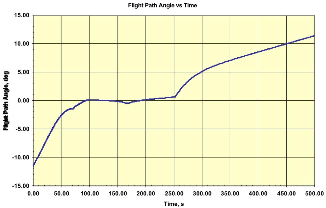
Figure 6-5 Taxi Mars Aerocapture Flight Path Angle Profile
