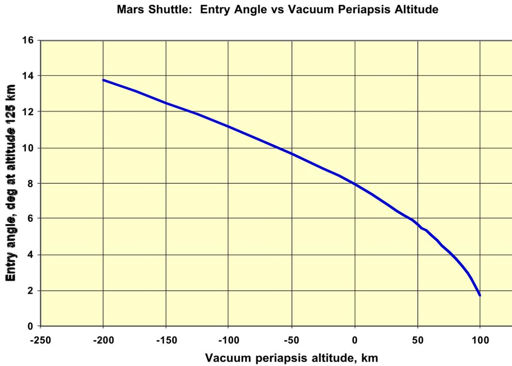
Figure 6-9 Entry Angle vs. Vacuum Periapsis Altitude for Entry from Phobos Orbit Radius
