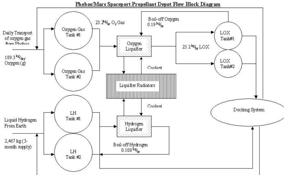
Figure 7-7: Mars Spaceport Propellant Depot Flow Block Diagram.
