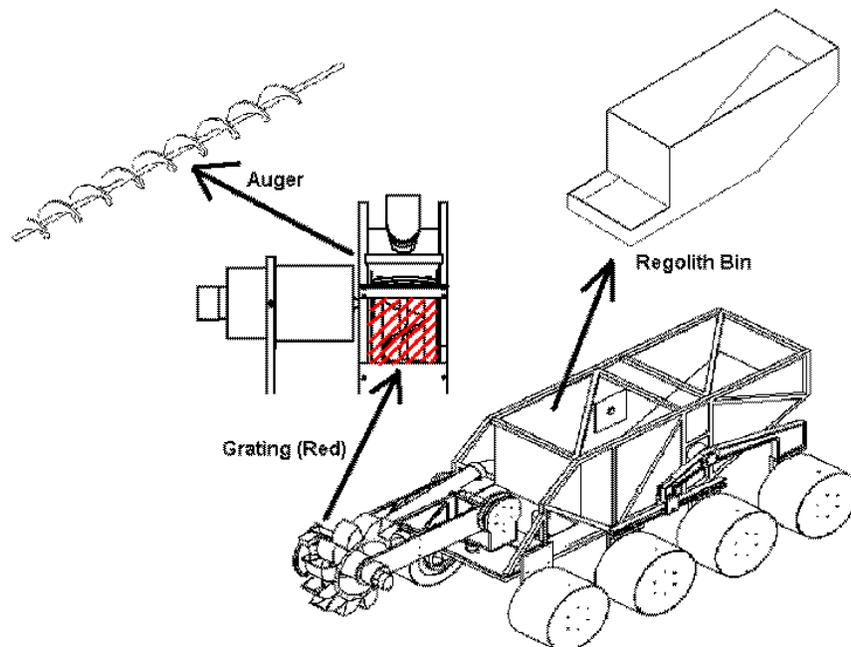
Figure 7-1 Prototype Mars Bucket-Wheel Excavator Design [35]
