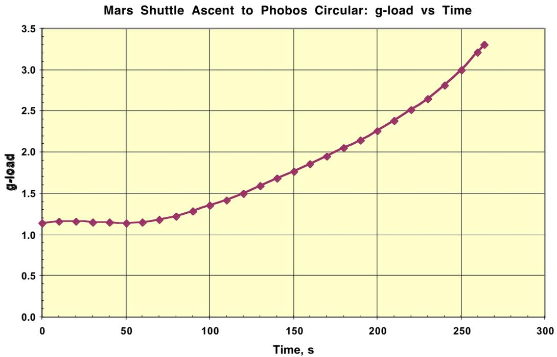
Figure 6-28 Ascent g-load versus Time
