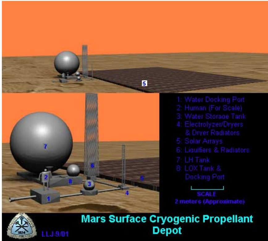
Figure 7-10 Mars Base Propellant Depot Rendered 3D Solid Model.
