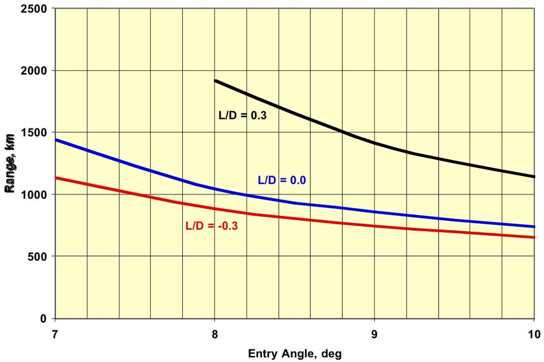
Figure 6-13 Range as a Function of Entry Angle
