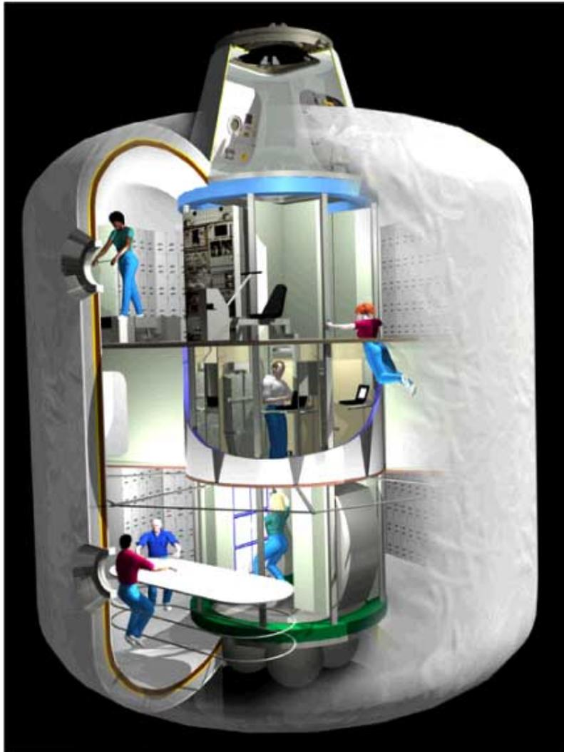
Figure 8-13 TransHab Design Cutaway (courtesy NASA/JSC)
