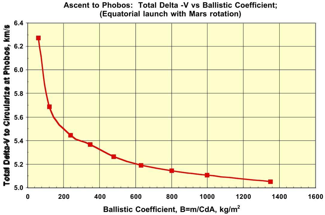
Figure 6-25 Delta-V versus Ballistic Coefficient
