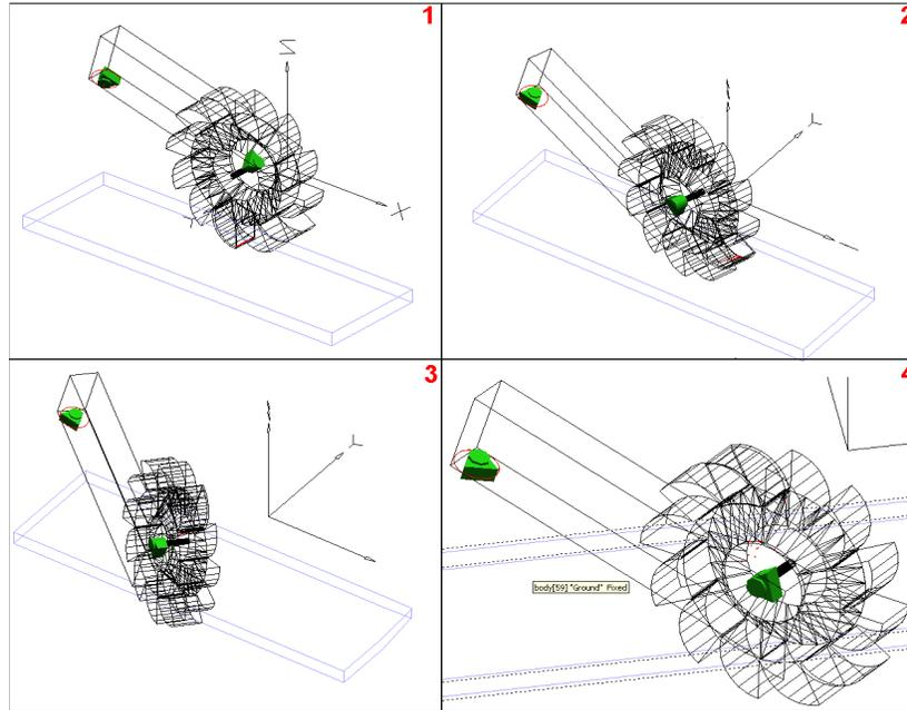
Figure 7-4 Bucket-Wheel/Boom & Regolith Particles Model.
