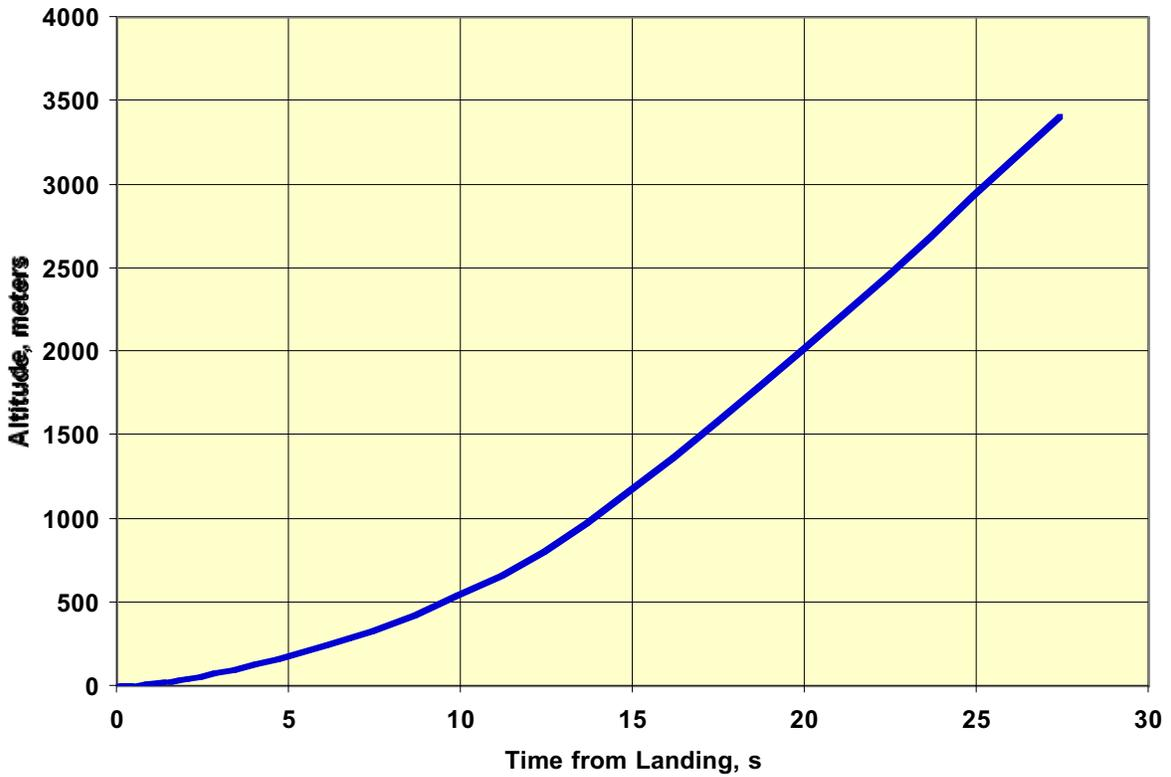
Figure 6-22 Altitude vs. Time for Entry Angle 8°, Deceleration of 1.5 gee, Beginning at 6 km.
