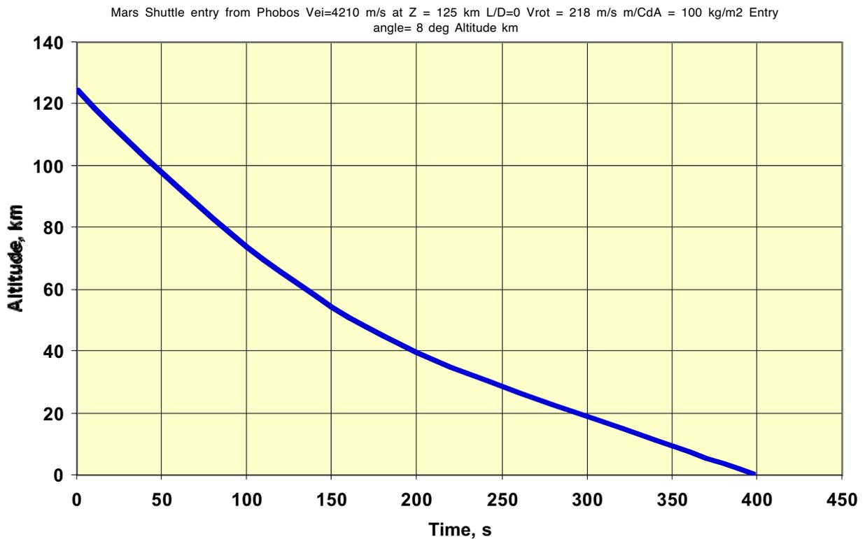
Figure 6-15 Mars Shuttle Entry: Altitude vs. Time
