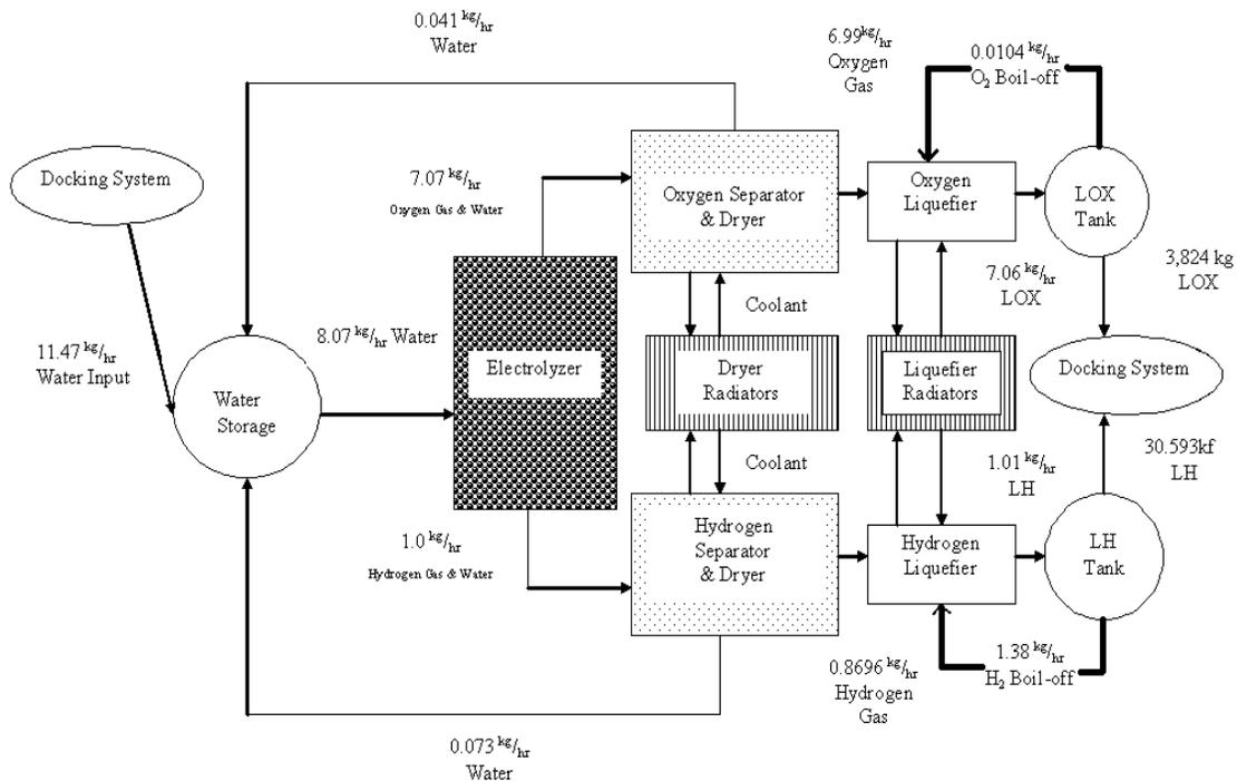
Figure 7-9: Mars Base Propellant Depot Flow Block Diagram.
