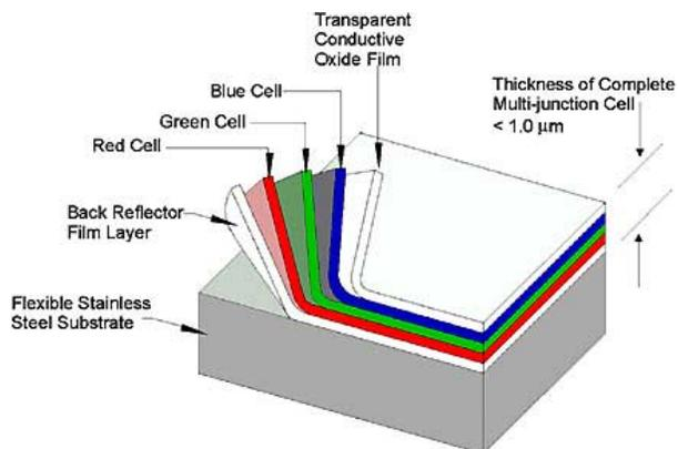
Figure 8-8 Triple Junction a-Si Cell
