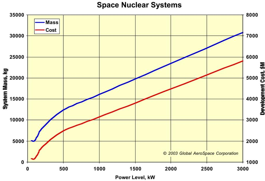
Figure 8-9 Space Nuclear Reactor System Mass and Cost as a Function of Power Level
