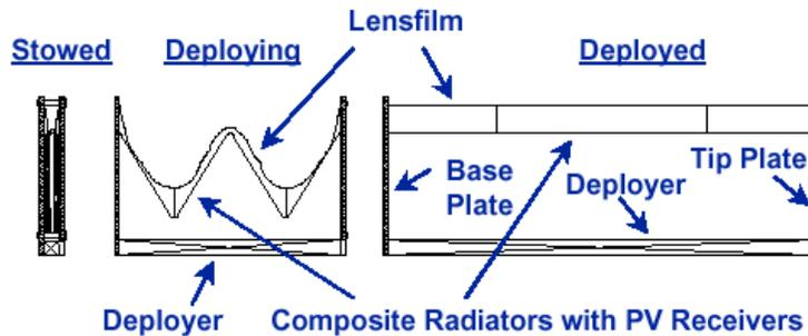
Figure 8-6 SLA Deployment Concept (Courtesy ENTECH)
