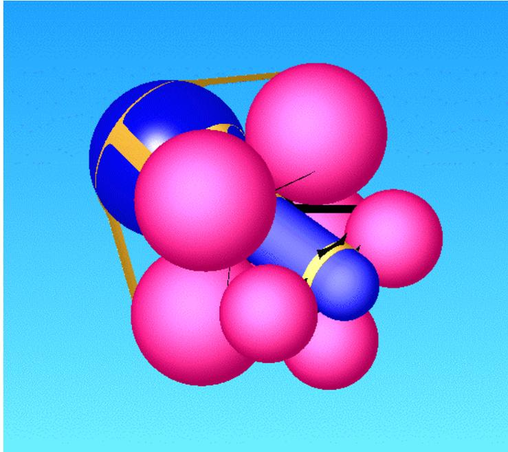
Figure 8-20 Propellant Augmentation Tanks for 1st and 2nd Taxi Stages
