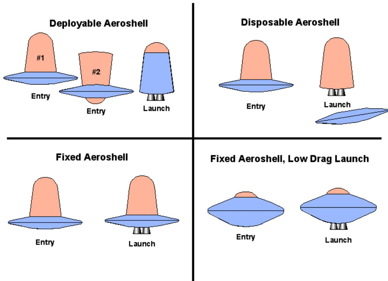
Figure 8-27 Mars Shuttle Entry and Launch Aeroshell Options
