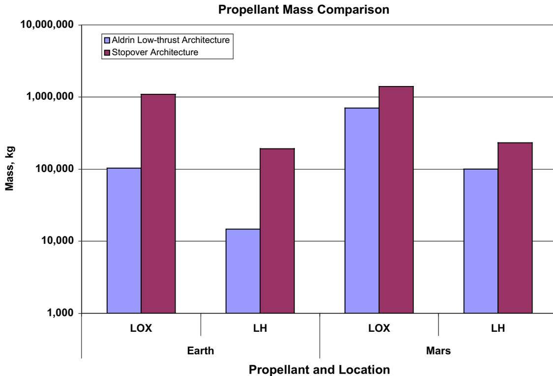
Figure 4-8 Propellant Mass and Location Requirements Comparison
