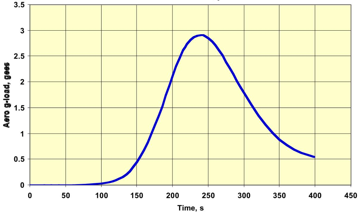
Figure 6-16 Mars Shuttle Entry: Aerodynamic g-load vs. Time
