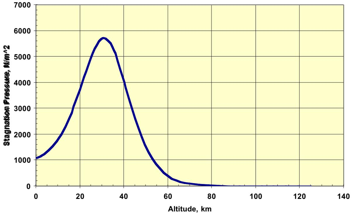
Figure 6-20 Mars Shuttle Entry: Stagnation Pressure vs. Altitude
