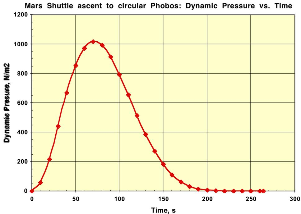
Figure 6-30 Ascent Dynamic Pressure versus Time
