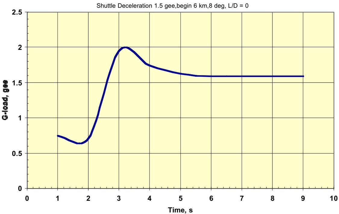
Figure 6-24 Deceleration g-load vs. Time from Landing for 1.5 Gee, 8° Entry Angle, Beginning at Altitude 6 km
