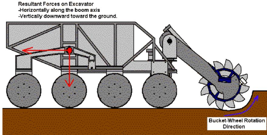
Figure 7-2: BWE Excavation Reaction Forces.
