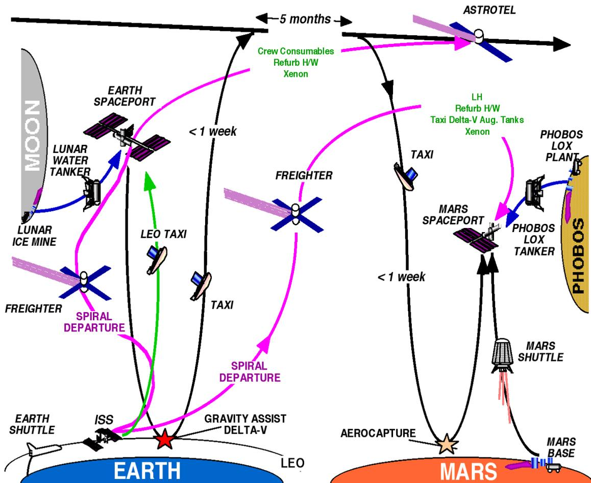
Figure 4-4 Aldrin Low-thrust Cyclers Mars Transportation Architecture Schematic
