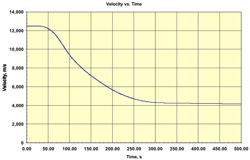
Figure 6-4 Taxi Mars Aerocapture Velocity Profile
