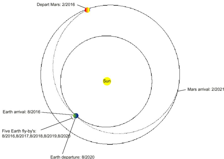
Figure 5-4 Example Semi-Cycler Showing Earth and Mars at Departure and Arrival Times (R. H. Bishop, et al, Earth-Mars Transportation Opportunities, Paper AAS 00-255)
