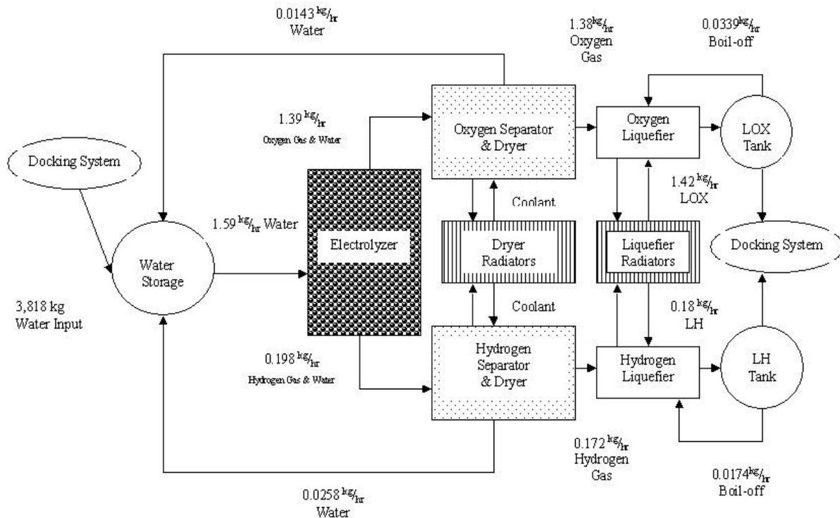
Figure 7-14 Earth Spaceport Propellant Depot Flow Block Diagram.
