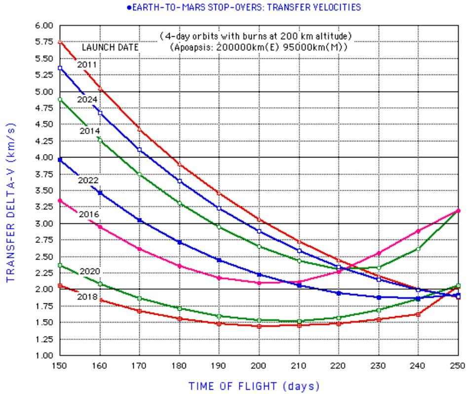
Figure 5-5 Delta-V versus Flighttime for Earth-to-Mars Stopover Trajectory Opportunities
