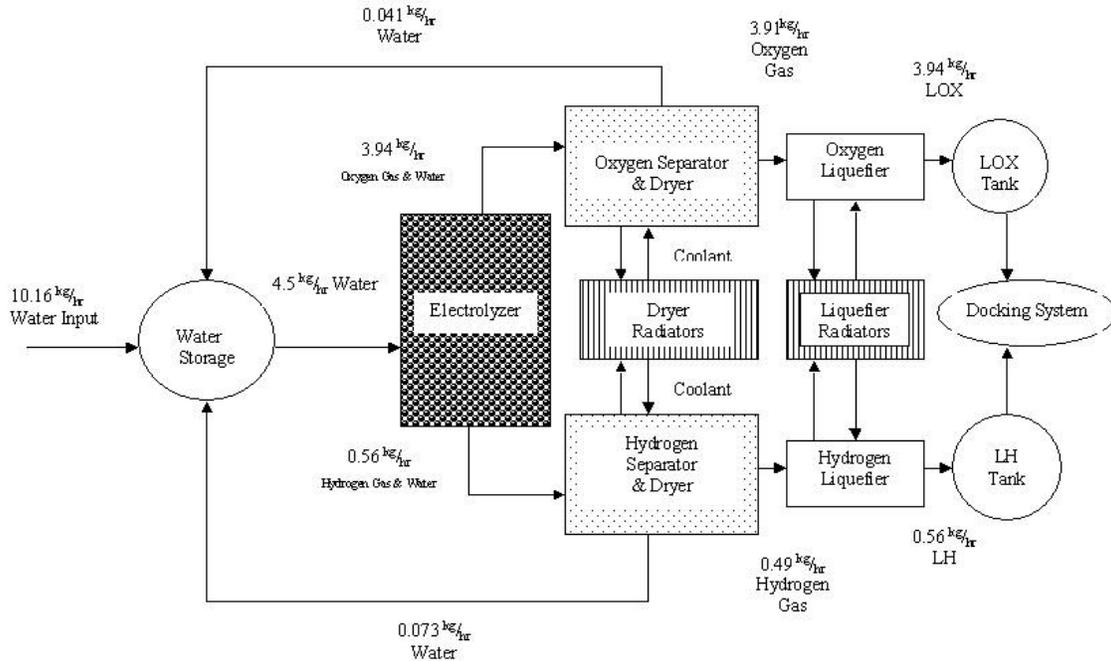
Figure 7-12 Lunar Polar Propellant Depot Flow Block Diagram.
