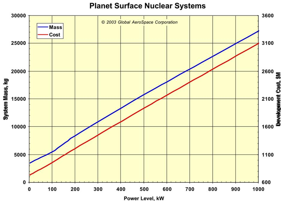
Figure 8-10 Surface Nuclear Reactor System Mass and Cost as a Function of Power Level
