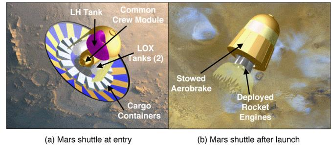
Figure 9 Mars Shuttle Configuration
