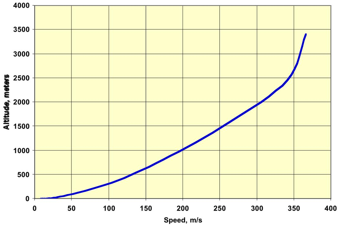
Figure 6-23 Altitude vs. Atmosphere Relative Speed for Deceleration of 1.5 gee, Beginning at 6 km, Entry Angle 8
