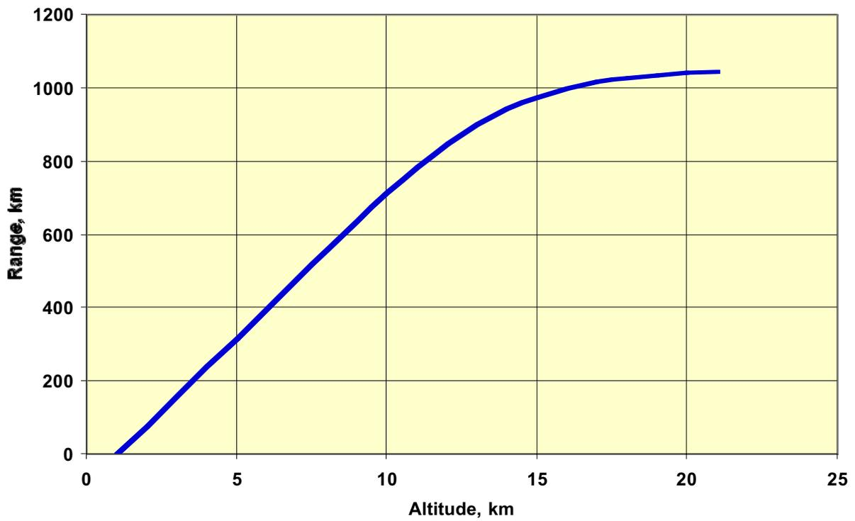
Figure 6-18 Mars Shuttle Entry: Range vs. Altitude
