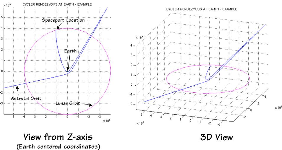
Figure 5-12 Example Hyperbolic Rendezvous from Lunar Orbit Radius in 3D
