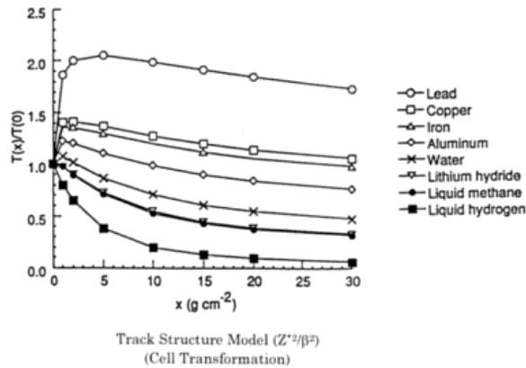
Figure 8-11 Required Shielding of Various Materials
