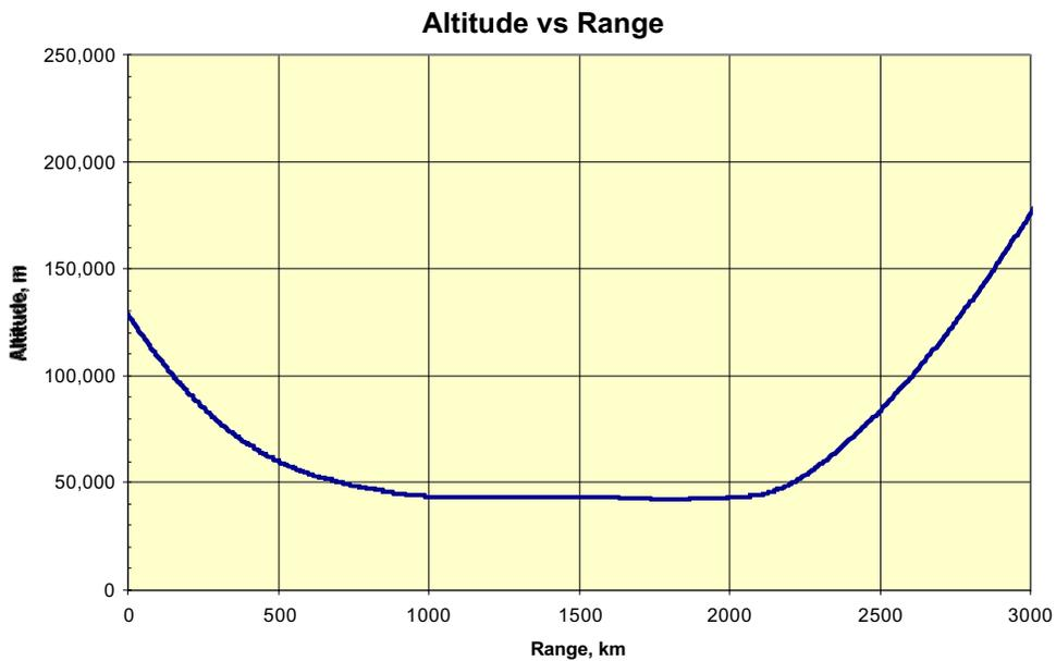
Figure 6-3 Taxi Mars Aerocapture Altitude vs. Range Profile
