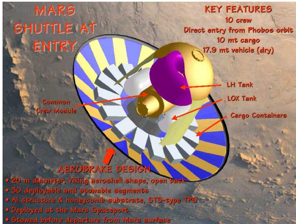
Figure 8-28 Mars Shuttle Aeroshell Design Concept
