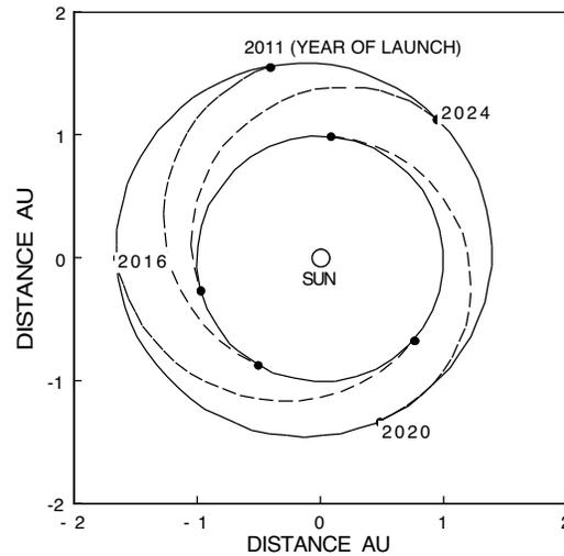
Figure 5-10 Astrotel 2 Mars-to-Earth Transfers
