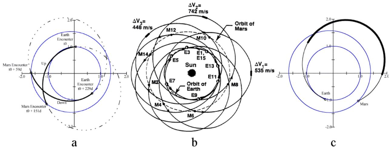
Figure 4-2 Aldrin Cycler Orbits: (a) Up and Down Escalators, (b) a 15-year Ballistic Up Escalator Sequence, (c) Example low-thrust orbit rotation augmentation maneuver
