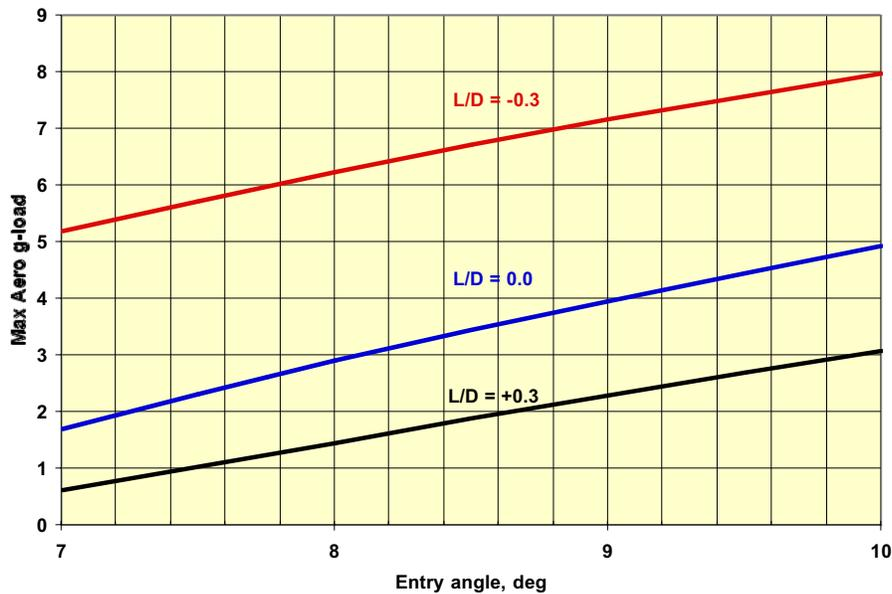
Figure 6-12 Maximum Aerodynamic  $g$ -load as a Function of Entry Angle
