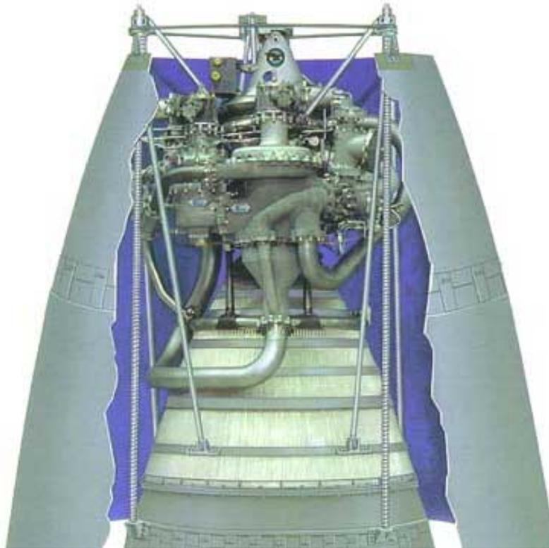
Figure 8-1 Pratt & Whitney RL10B-2 Engine
