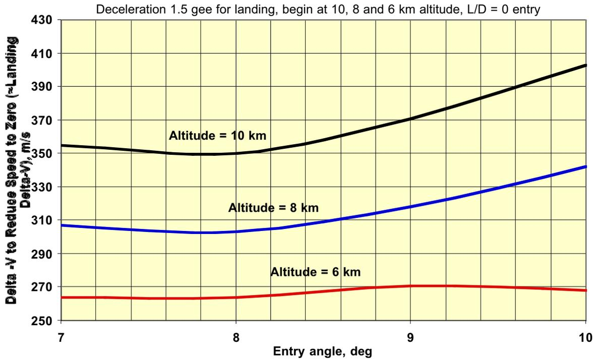
Figure 6-21 Landing Delta-V vs. Entry Angle and Burn Start Altitude
