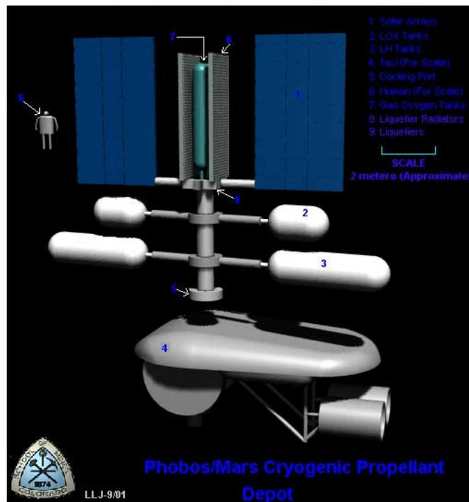
Figure 7-8: Mars Spaceport Propellant Depot Rendered 3D Solid Model.
