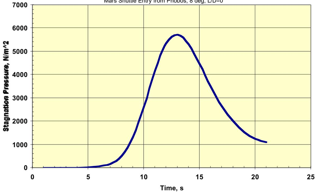
Figure 6-17 Mars Shuttle Entry: Stagnation Pressure vs. Time
