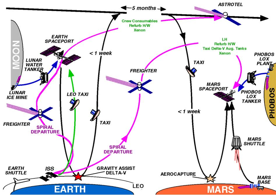
Figure 1-2 Mars Transportation Architecture Schematic
