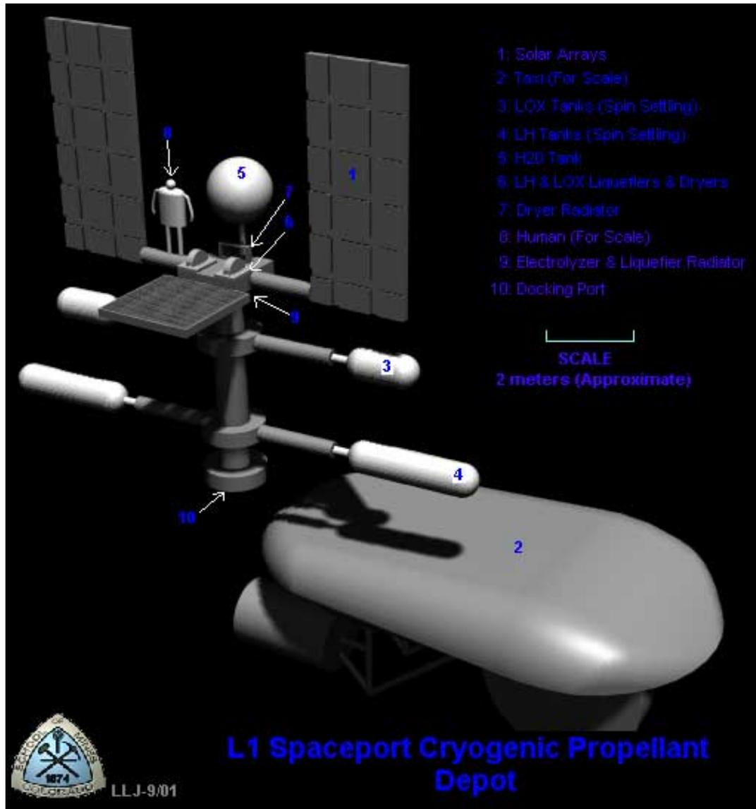
Figure 7-15 Earth Spaceport Propellant Depot Rendered 3D Solid Model.
