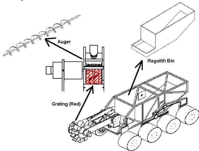
Figure 10 Bucket Wheel Excavator and Transporter
