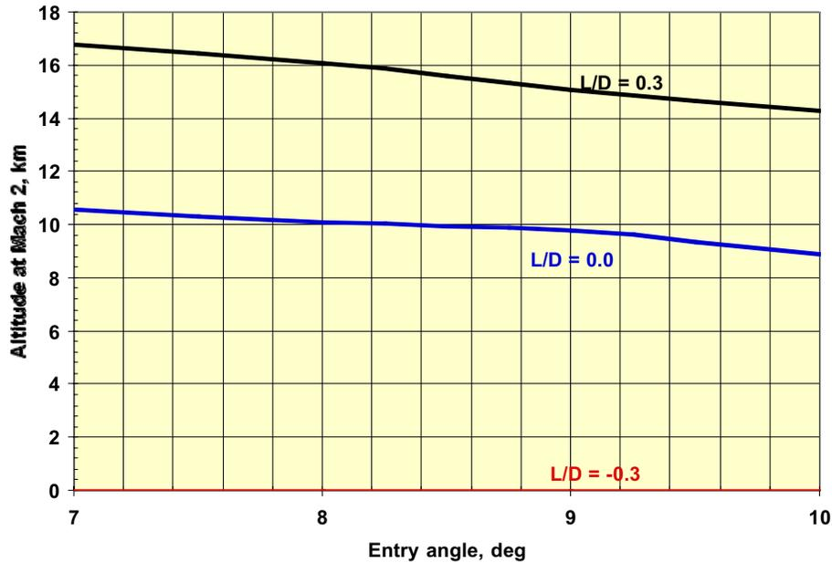
Figure 6-11 Altitude at Mach 2 as a Function of Entry Angle
