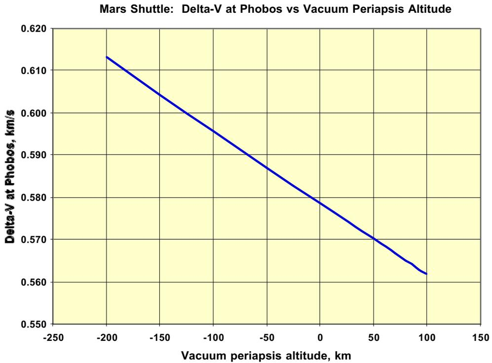
Figure 6-10 Delta-V at Phobos Orbit Radius vs. Vacuum Periapsis Altitude
