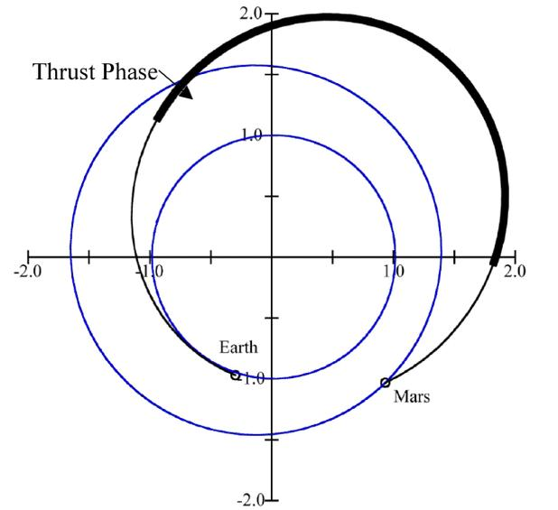
(a) Astrotel Low-thrust orbit shaping
