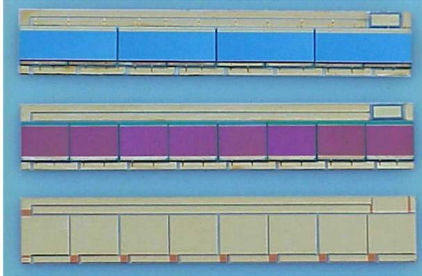
Figure 8-7 Example of a Stacked Cell Set (Courtesy JX Crystals)
