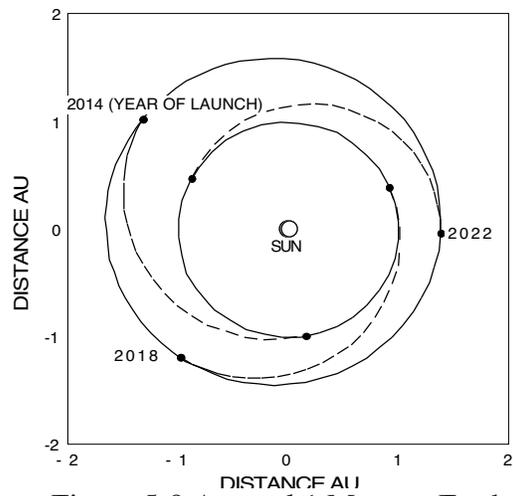
Figure 5-9 Astrotel 1 Mars-to-Earth Transfers
