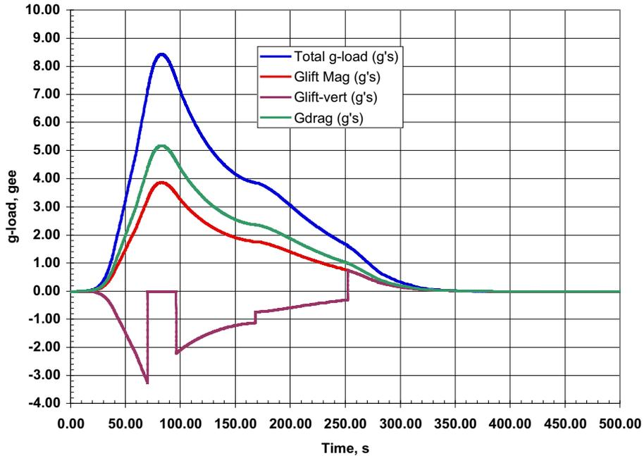
Figure 6-8 Various components of g-load vs. Time
