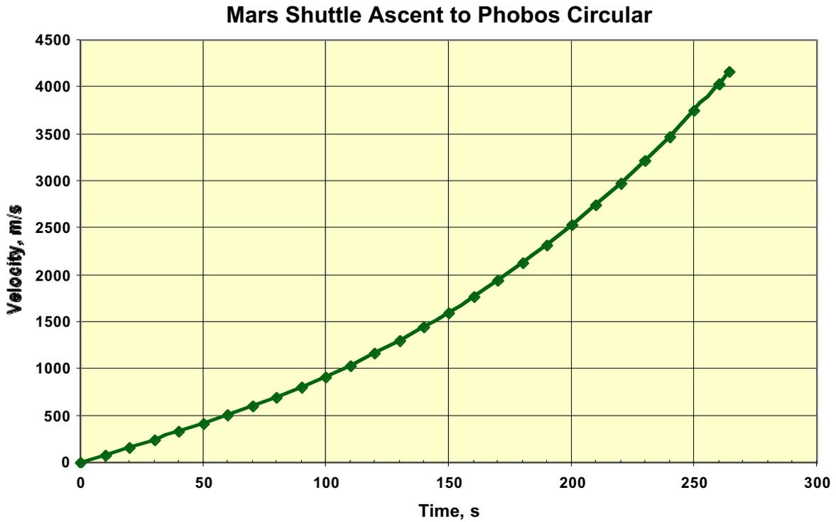
Figure 6-27 Ascent Velocity versus Time
