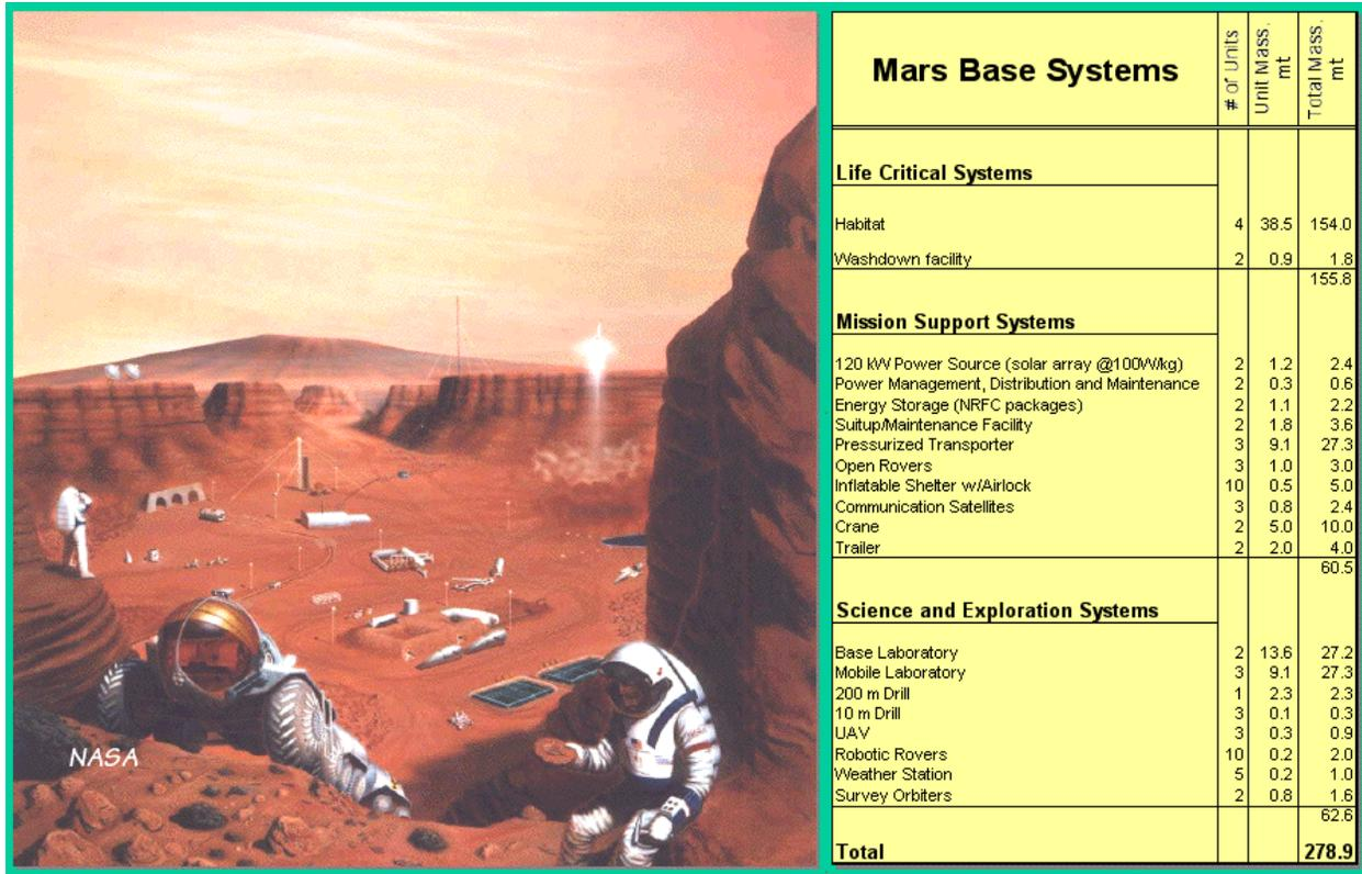
Figure 4-1 Mars Base Concept and Equipment Inventory
