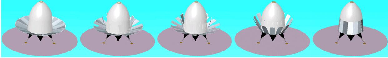
Figure 8-29 Mars Shuttle Aeroshell Stow Sequence
