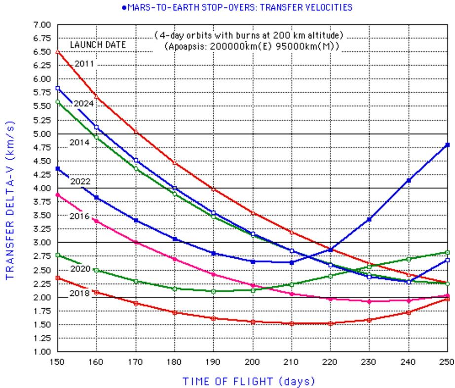
Figure 5-6 Delta-V versus Flighttime for Mars-to-Earth Stopover Trajectory Opportunities
