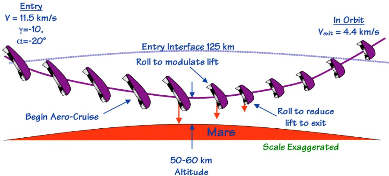
Figure 6-1 Schematic of Aerocapture Maneuver at Mars
