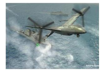
Tern — a program to give forward-deployed small ships the ability to serve as mobile launch and recovery sites for medium-altitude, longendurance unmanned aerial systems— has just entered the second phase, with AeroVironment Inc. and Northrop Grumman Corp. the prime contractors.
