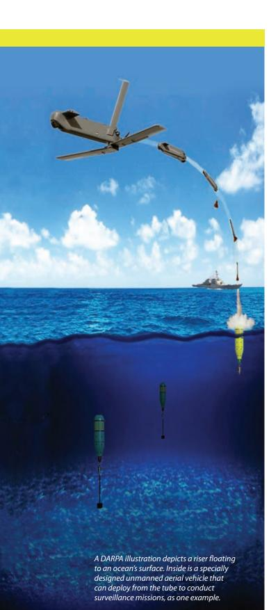
mission node capable of launching a payload from a depth of more than 6 kilometers (3.7 miles). "By exploiting environmental conditions and basic physics, it is anticipated that the riser and the UAV will enable powerful effects with a large influence range at low cost and risk," says a GAC statement about the company's contribution to the DARPA-led effort.
